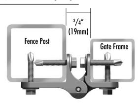
**NOTE:** Kwik-Fit hinges are intended for post mounting only. For mounting to walls where there is no room for a fence post, use D&D's "Multi-Adjust" MFA model.
